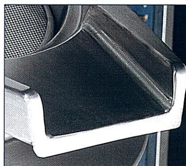
Seamless welded tank
